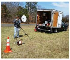
USGS scientist calibrates an electromagneticinduction borehole probe as part of the geophysical data collection at monitoring wells on Shinnecock Nation Tribal Lands. Photo credit: USGS
