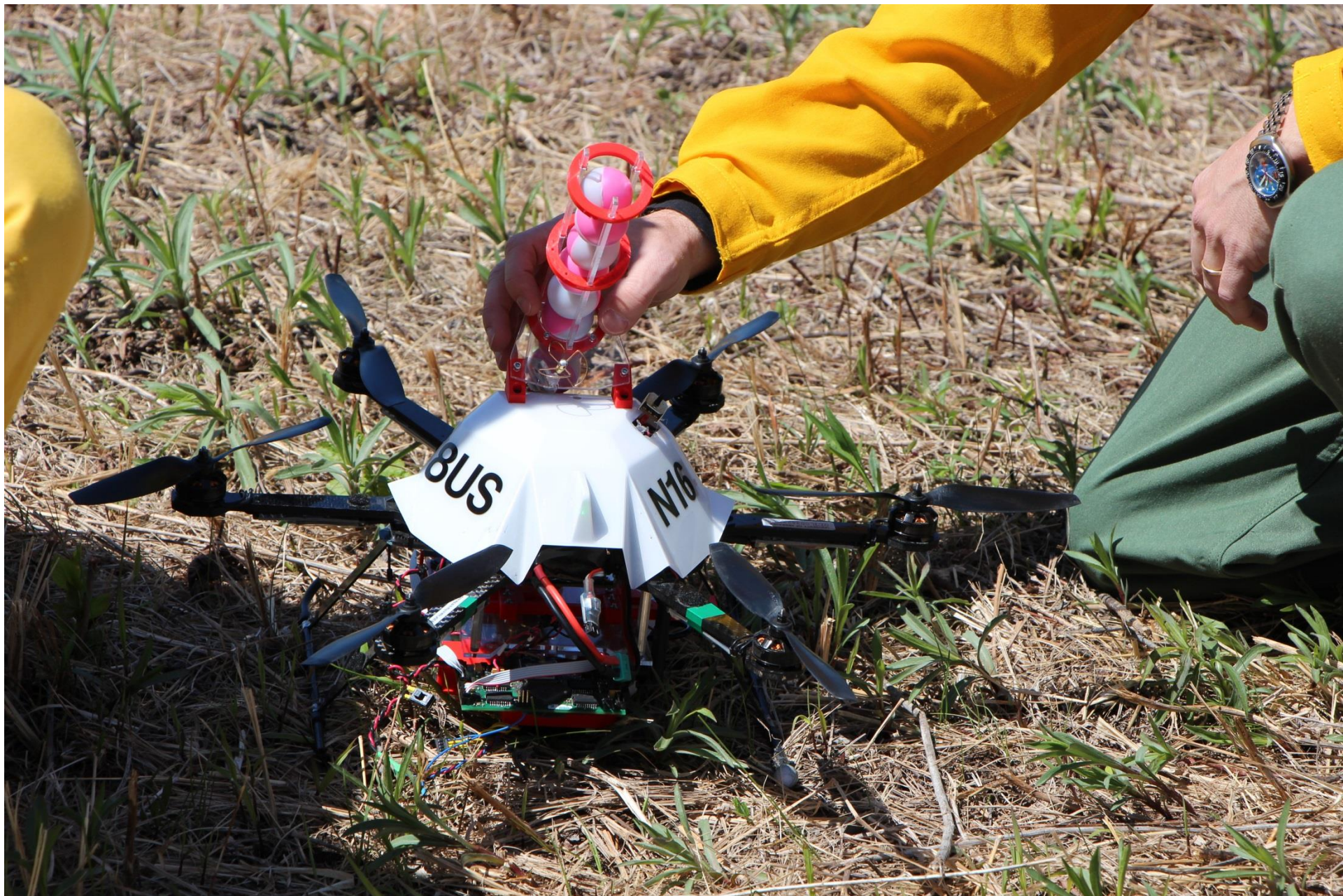
Img_6505.jpg – The small unmanned aircraft system loaded and ready to inject liquid into the plastic spheres so they can be injected and dropped to start the interior portion of the prescribed fire. Photo Credit NPS Volunteer Robin Matty
