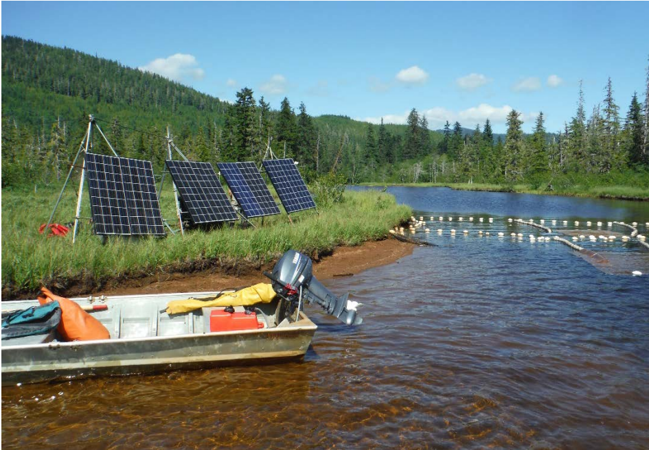
Figure 2. View of the solar panel array and net weirs at the Sitkoh Lake video weir.
