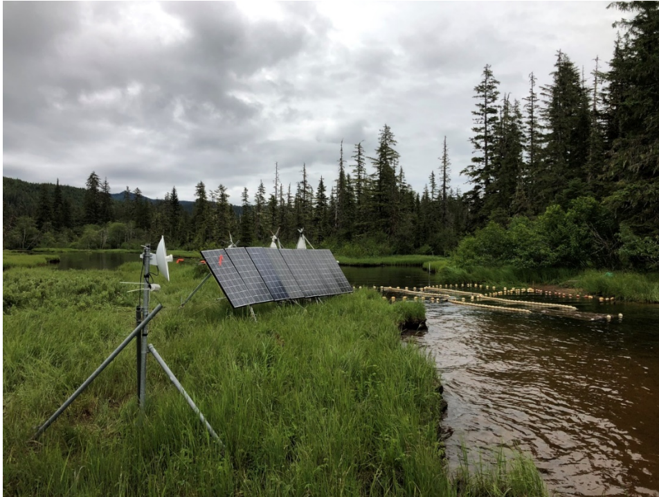
Figure 2. The video weir at the outlet of Sitkoh Lake, July 9, 2020.
