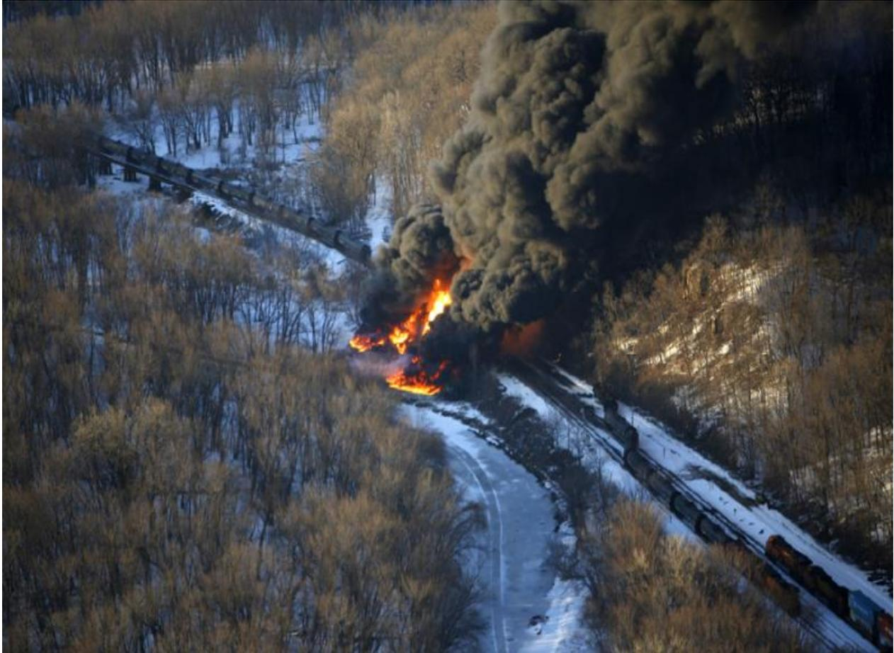
**Response to Crude-by Rail spill: In March 2015, 21 cars of a 105 tank-car shipment of crude oil derailed near Galena, IL. Five of the derailed cars caught fire and ruptured, releasing oil onto an embankment and wetland adjacent to the Galena River and just upstream of the Mississippi River. Potential impacted resources included the adjacent Upper Mississippi National Wildlife Refuge. Representatives from the FWS responded to the spill. (U.S. EPA photo)**
