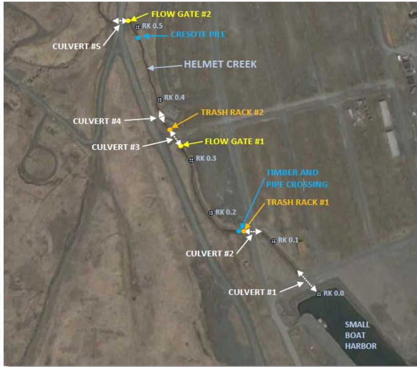
Figure 1: Lower Helmet Creek showing structures
