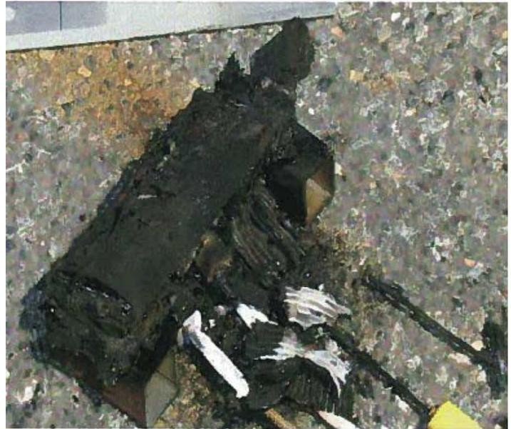
By comparison to standard alkaline batteries, most lithium-ion batteries manufactured today contain a flammable electrolyte with a very high energy density. A lithium battery is susceptible to thermal runaway, a destructive chain reaction resulting from self-heating and the release of its stored energy.
