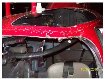
Minerals Management Service (MMS) inspector was sitting. Part of the bird exited through the overhead skylight and struck the vertical fin. The bird inflicted damage to the windshield, windshield frame, skylight, vertical fin and...the inspector!
