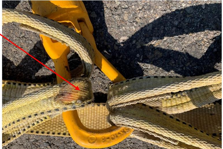
Faded areas, showing UV damage to straps
