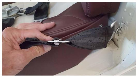
Compare the orientation of the webbing loop in the photo above...... to the PROPER WEBBING LOOP in diagram (a-1) from FAA Advisory Circular 21-34 below.
