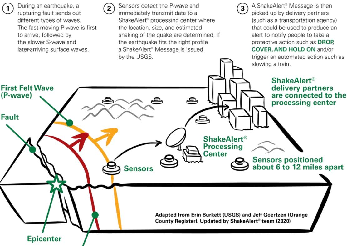
The graphic above describes the basics of how the *ShakeAlert* earthquake early warning system operates during an earthquake. Source: USGS.
