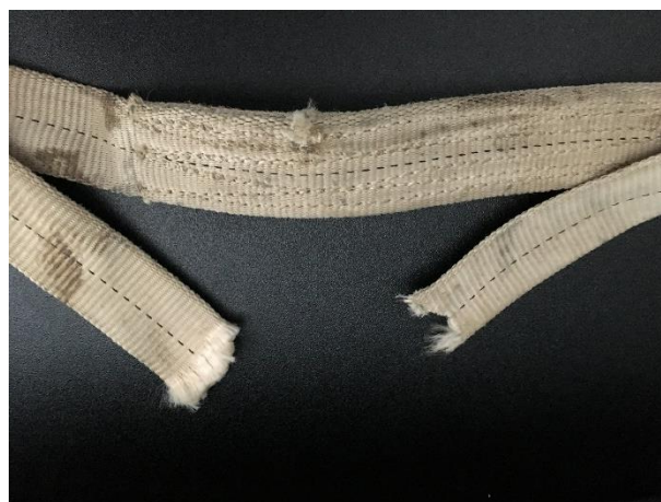
Figure 1 Abrasion Wear on Non-Commercial Choker Equipment
