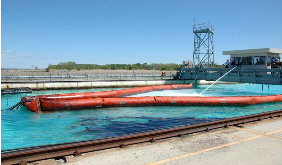
Figure 2. Ohmsett students training on the application of dispersants to an oil spill.
