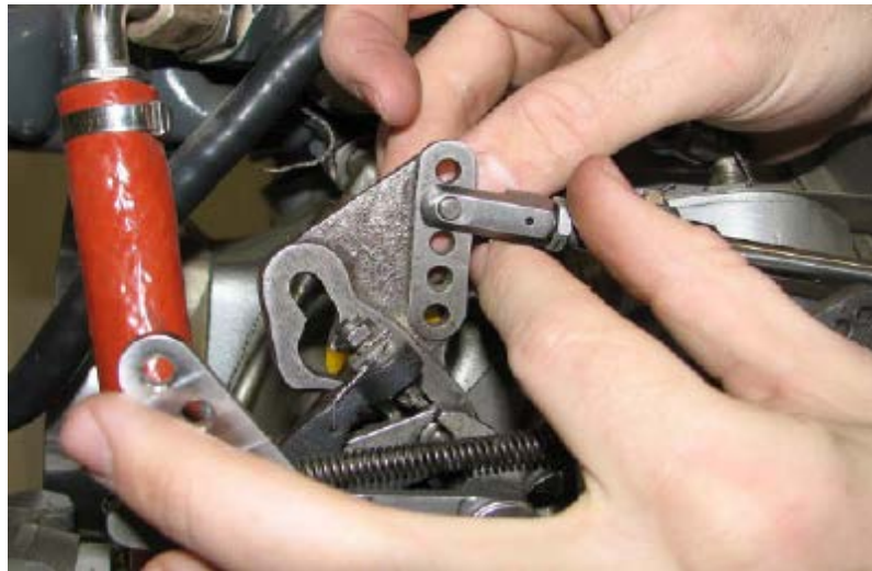
Figure 76-35 - Reinsert the Clevis Pin After Extending the Clevis 1/2 Turn
