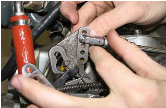
Figure 76-35 - Reinsert the Clevis Pin After Extending the Clevis 1/2 to 1 Turn
