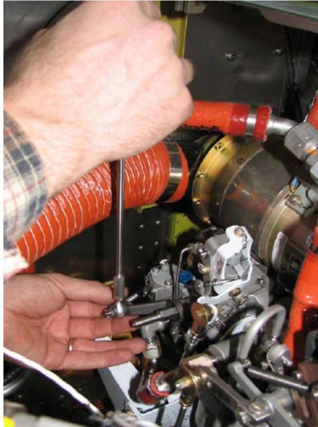
Figure 76-37 - Gently Feel for the FCU Arm Pick-Up Point
