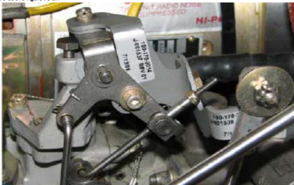
FIGURE 76-16 - Fuel Condition Lever at High Idle
