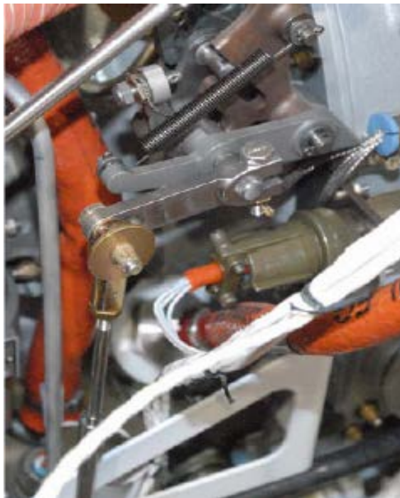
Figure 76-24 - Connect the Rod to the Outermost hole on the Cambox Lever
