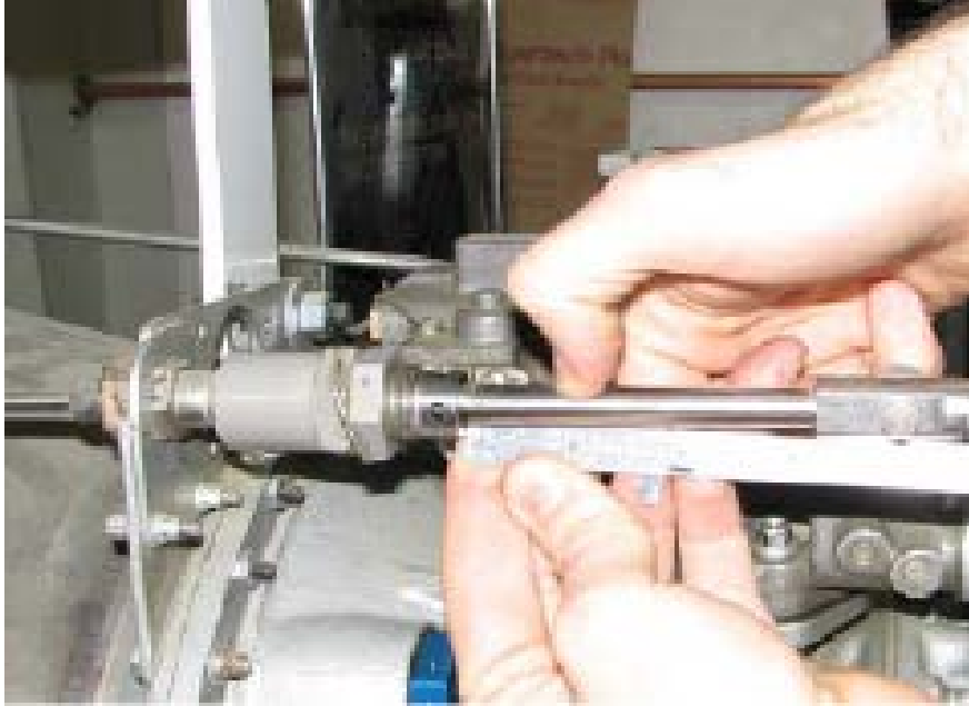
Figure 76-29 - Recheck Distance "L" with Cable Extended
