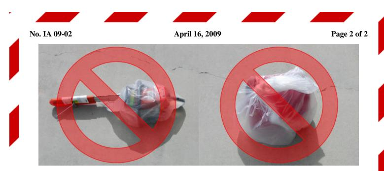
**3. Drip Torches.** Drip torches (1) must be transported with the igniter nozzle assembly in the tank, air breather valve closed, tank lockring sealed, and fuel spout plug closed and (2) must be secured in the upright position. Leave a minimum of 2 inches of air space below the container opening when filling.
