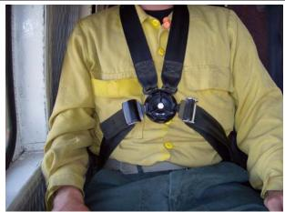
Figure 2 - Incorrectly fastened. This will not provide adequate protection in the event of a mishap.
