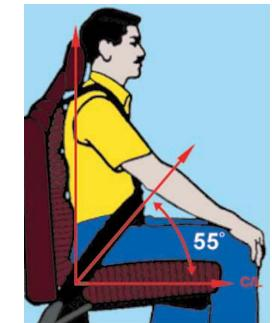
Figure 3 - The safety belt should be positioned so that it makes an angle of about 55 degrees with the centerline of the aircraft.
