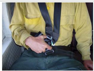
Figure 4 - Incorrectly fastened. The whole center section turns, not just the release. This may delay egress.
