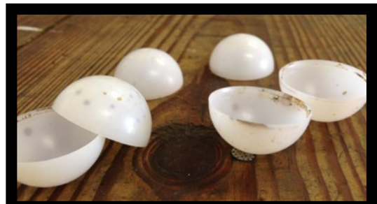
Figure 4. Loose Aerostat (PSDS) sphere halves. Potassium permanganate residue is visible on the sphere surfaces.
