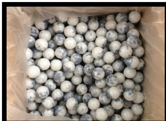
Figure 2. SEI's Premo spheres with a spotted appearance on the internal surface. Some of VPL's Premo spheres also have a spotted appearance (figure 1).
