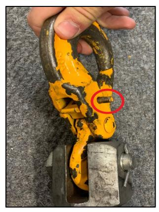
Figure 1. Esmet Swivel showing protruding roll pin.
