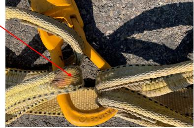
Faded areas, showing UV damage to straps
