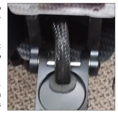
4. Locate **the foam plug and** gently pull the cable through. This will expose four screws that go in to the motor base. With a magnifying glass and light, inspect the area around each bolt head for signs of cracks or defects.
