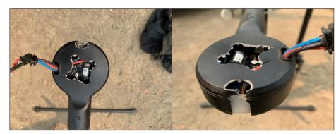
Figure 2: Motor mount after departure of motor.
