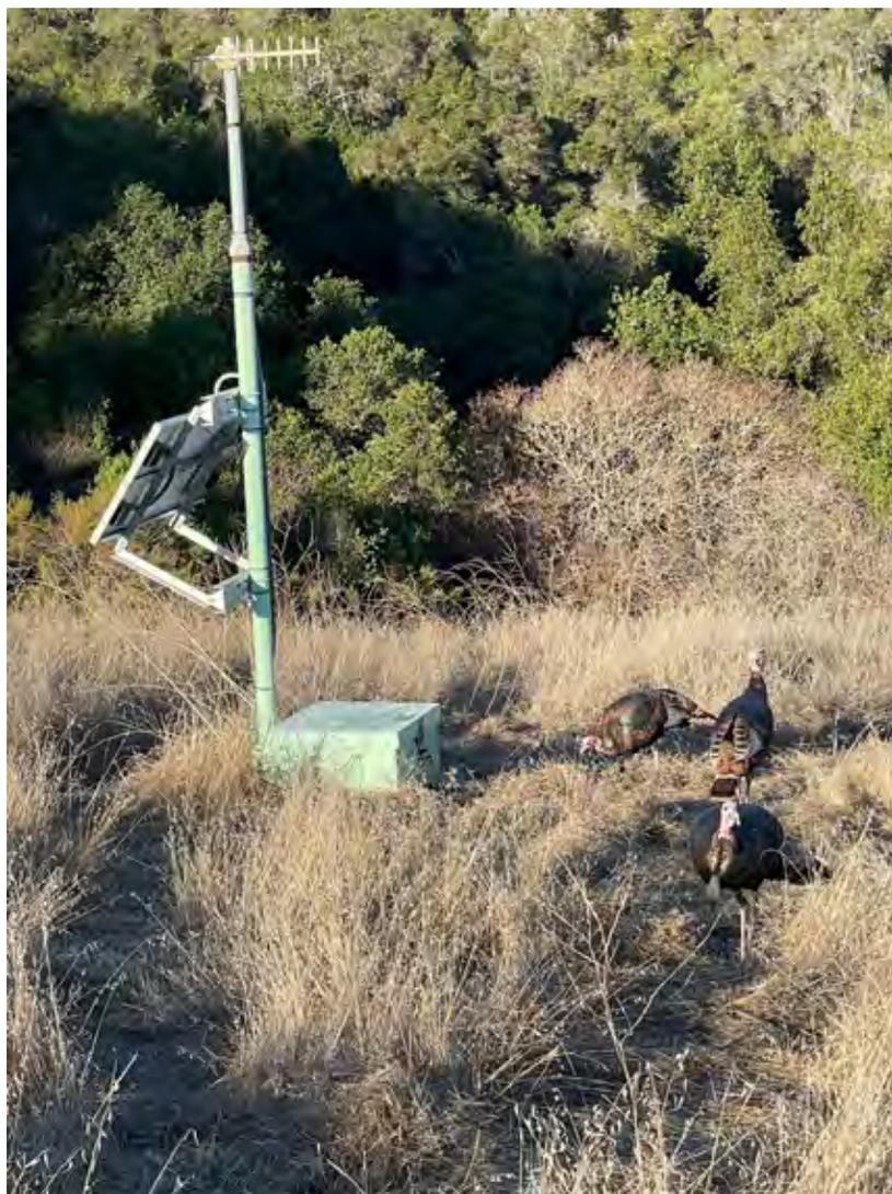
Earthquake early warning system monitoring station.
