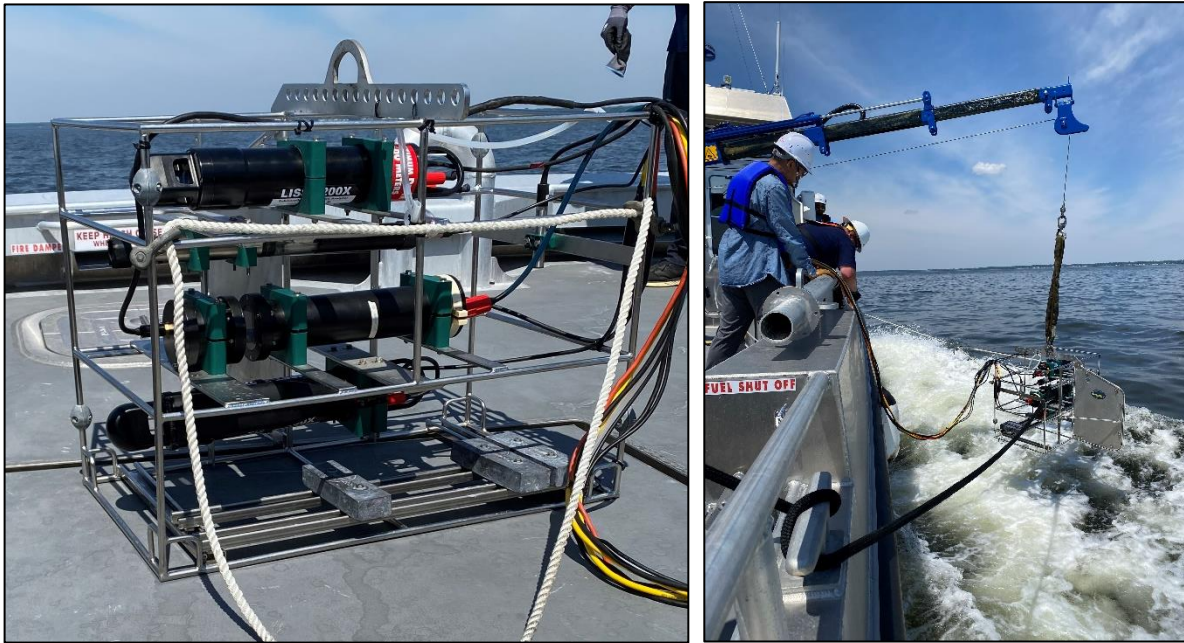
FIELD EVALUATION OF SURFACE WATER DISPERSANT MONITORING USING DSD INSTRUMENTATION AND INSTRUMENT CARRIAGE SYSTEM. THIS RESEARCH INVESTIGATES HOW AVAILABLE TECHNOLOGY CAN SUPPORT OIL SPILL PREPAREDNESS AND RESPONSE ACTIVITIES. SOURCE: BSEE
