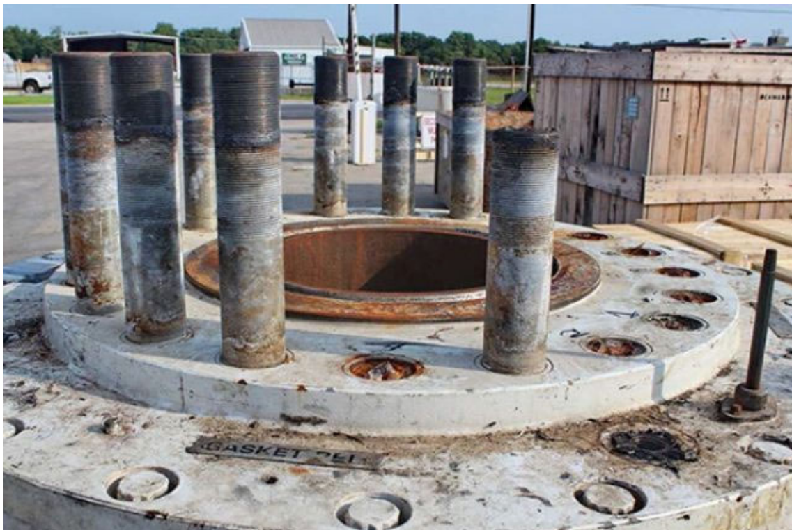
FAILED BOLTS IN A HYDRAULIC CONNECTOR AFTER ONLY 4 MONTHS IN SERVICE AT 5,720 FEET OF WATER DEPTH. THIS CONNECTOR IS DESIGNED TO LINK A LOWER MARINE RISER PACKAGE AND A LOWER BLOWOUT PREVENTER, WHICH PREVENTS THE UNCONTROLLED DISCHARGE OF HYDROCARBONS FROM A WELL. PHOTO: BSEE QC-FIT REPORT #2016-04, FEBRUARY 2016.
