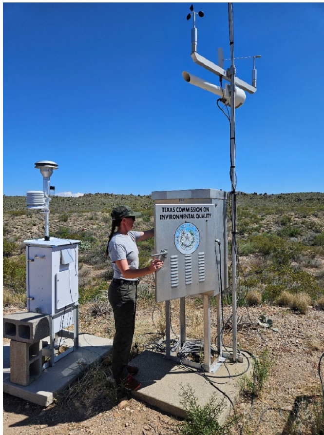
NPS SITE OPERATOR KELON CRAWFORD PERFORMS MONTHLY VERIFICATIONS ON THE CAMS 316 MONITORING STATION IN BIG BEND NATIONAL PARK. IN FY2023, THIS STATION COLLECTED DATA ON AIR POLLUTION; WIND SPEED, DIRECTION, GUST, AND STANDARD DEVIATION OF HORIZONTAL WIND DIRECTION; AND OUTDOOR TEMPERATURE. PHOTO: NPS/STAFF.
