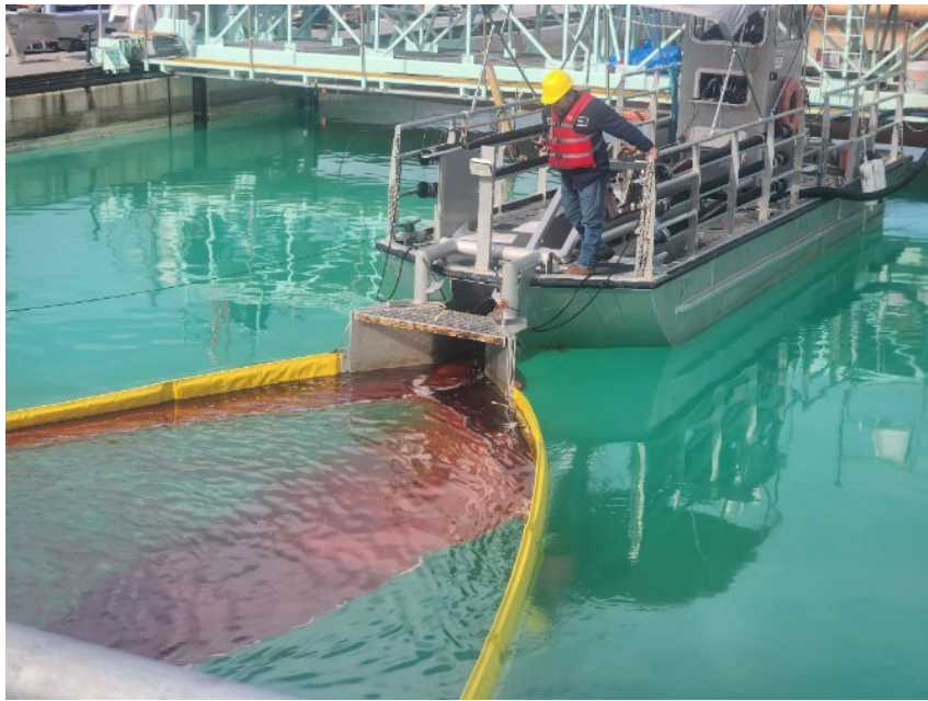
ELASTEC KVICHAK VESSEL WITH AN X30 GROOVED DISC SKIMMER COLLECTING DIELECTRIC FLUID IN A TEST POOL. THIS TECHNOLOGY IS DESIGNED TO HELP RECOVER POLLUTANTS DISCHARGED FROM OFFSHORE WIND TURBINES. PHOTO: BSEE
