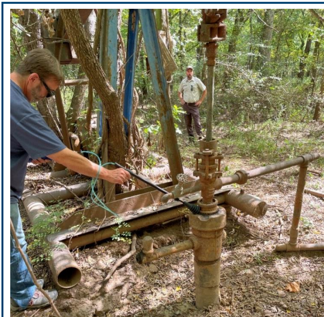
Figure 41. Using equipment to conduct a methane detection test at an orphaned well in a National Wildlife Refuge.
