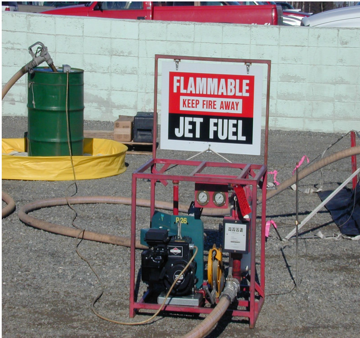
Figure 3 Alaska Fire Service Dispensing Module: Gasoline engine powered pump (shielded ignition, spill plate, spark arresting muffler, filter, meter, bonding wire, hose, dispensing nozzle, etc.).
