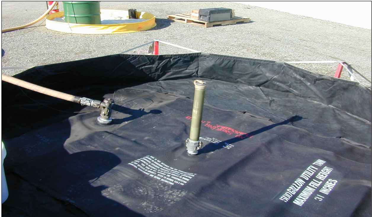
Figure 1 Alaska Fire Service 500-gallon bladder set up in a containment dike.
