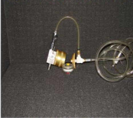
FIG 4.2 GTP-7 SAMPLING CONNECTION
