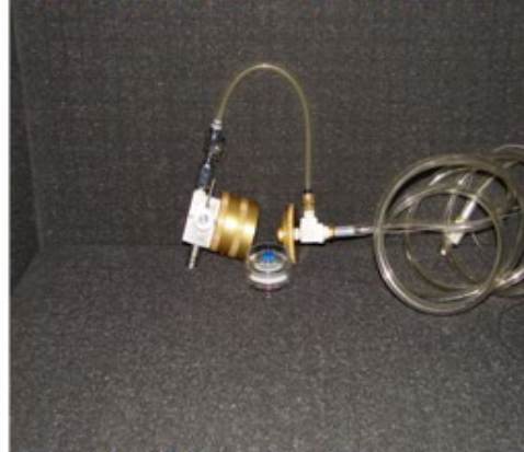
FIG 4.3 GTP-7 SAMPLING CONNECTION
