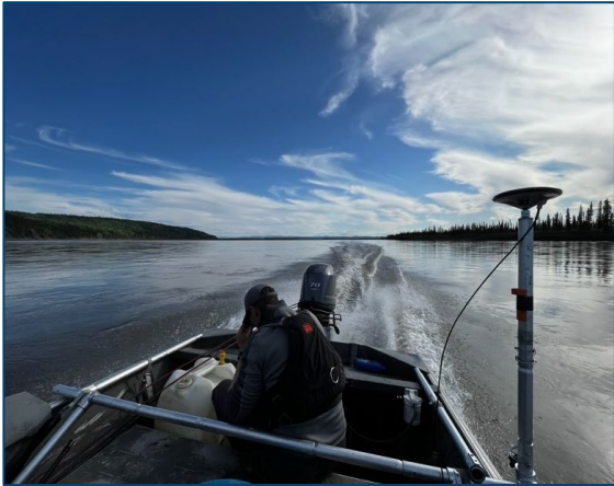
Photo, surface water gage equipment mounted on a river boat on the Yukon River, by Tamlin Pavelsky.
