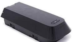
This test highlighted a safety of flight issue when the batteries are approaching 35%. As a result, 3DR solo batteries should not be flown below that threshold and flights should plan to terminate prior to reaching the 35% limitation. Landing battery levels should also be recorded on field forms to document and ensure compliance with this revised safety practice.
