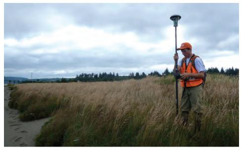
A USGS technician collects critical elevation data using a Real-Time Kinematic Global Positioning System at the Bandon National Wildlife Refuge, managed as part of the Oregon Coastal Refuge Complex, in southern Oregon. Photo credit: Katherine Powelson, USGS
