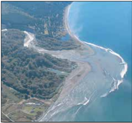
Aerial photo of the Elwha River mouth and expansion of the river mouth delta by sediment deposition as a result of removing upstream dams. Photo credit: Neal and Linda Chism of LightHawk
