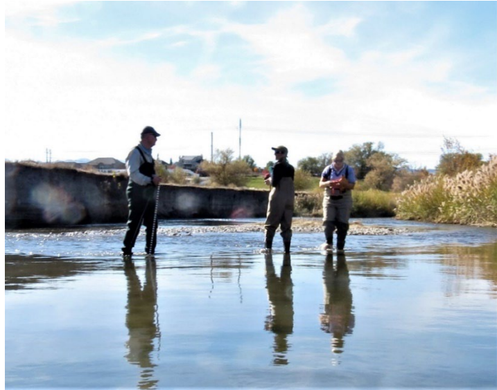
Community Scientists collect river cross-section measurements (Photo: Dan Potts)
